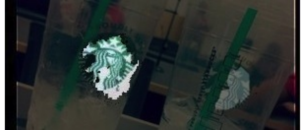
Figure 1: The two highlighted Starbucks logos are partially recognized by NRDC as visual words.
