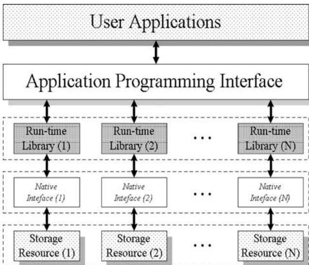
Figure 3. Logic architecture of multi-storage resource system.
