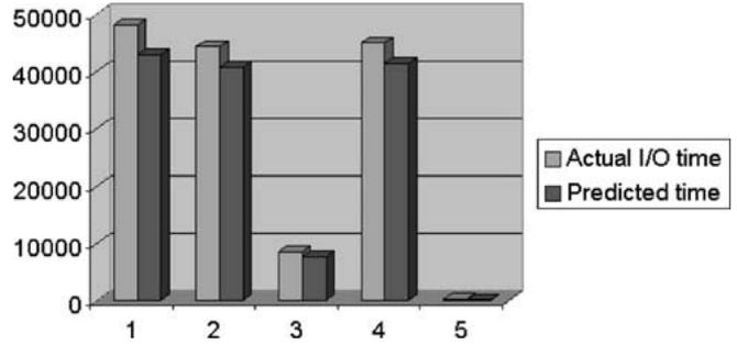
Figure 9. I/O time for Astro3D: (1) write all datasets to remote tapes; (2) write *temp* to remote disks and all other datasets to remote tapes; (3) write only *temp* to remote disks and *press* to remote disks; (4) write *vr-temp* to local disks and all the other datasets to remote tapes; (5) write only *vr-temp* to local disks and *vr-press* to remote disks.
