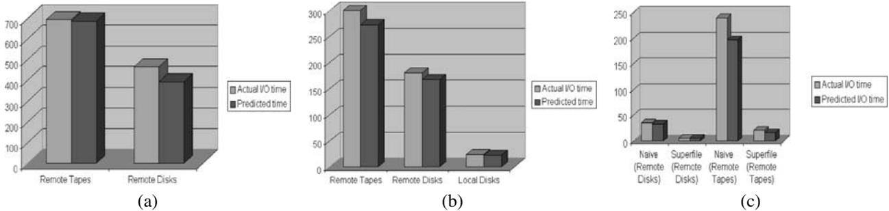
Figure 10. I/O time for data analysis (a), visualization (b) and superfile (c).
