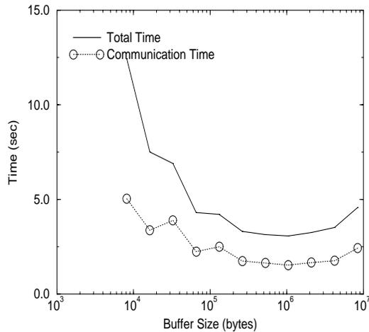
**Figure 3. Communication time and Total time taken by collective read operation (Array size=1024 X 1024, Distribution=column-block, Processors=32)**
