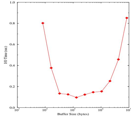
**Figure 2. I/O time taken by collective read operation (Array size=1024 X 1024, Distribution=column-block,Processors=32)**
