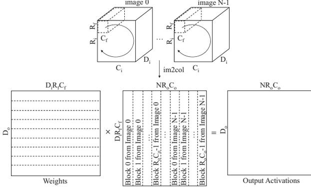
Figure 2: Computing activations using *im2col* at the first fully-connected layer.  $N$  images are transformed to a single matrix and the weight matrix is multiplied by the transformed matrix. The result is the output activations.
