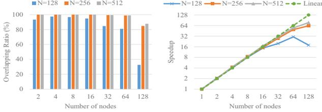
Figure 8: Overlapping ratio (left) and speedup (right) with varying mini-batch size.  $k$  is set to 9, and  $f$  is set to 2. The larger mini-batch size increases the computation workload and allows the higher overlapping ratio.
