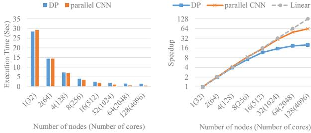
Figure 6: VGG-A training time (left) and speedup (right) for a single mini-batch size of 256.  $k$  is set to 9 and  $f$  is set to 2. We compare our approach (parallel CNN) with the pure data-parallel training algorithm (DP). The speedup is calculated with respect to the number of nodes.
