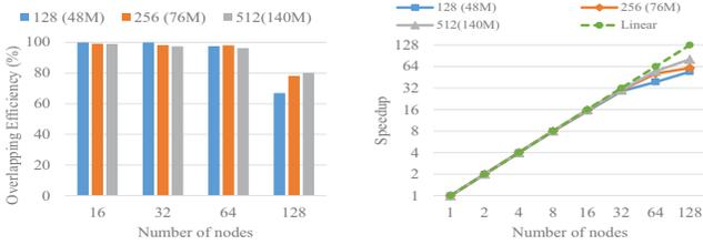
Figure 9: Overlapping ratio (left) and speedup (right) with varying number of parameters. VGG-128, VGG-256, and VGG-512 models are trained on a single mini-batch size of 256. Maximum speedups are  $54\times$ ,  $61\times$ , and  $80\times$  respectively.
