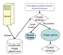
**Fig. 1**. Flow chart of a server side image spam detection system by cluster analysis.
