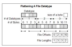
Figure 3: Example flattening of a file datatype. File datatypes are converted into lists of file offsets and lengths in order to generate the necessary parameters to use the list I/O interface.
