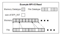
Figure 2: File datatypes are replicated and read into memory until the read call has accessed that correct amount of data.
