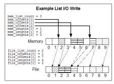
Figure 1: Example list I/O write. Since only contiguous regions can be described using the POSIX read/write interfaces, four I/O calls would be required instead of one list I/O write.
