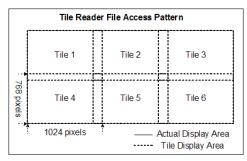
Figure 4: Tile reader file access pattern. Each processor is in charge of reading the data from a display file into its own local display, also known as a tile. This results in a noncontiguous file access pattern.
