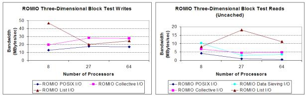
Figure 7: Three-dimensional block test results.
