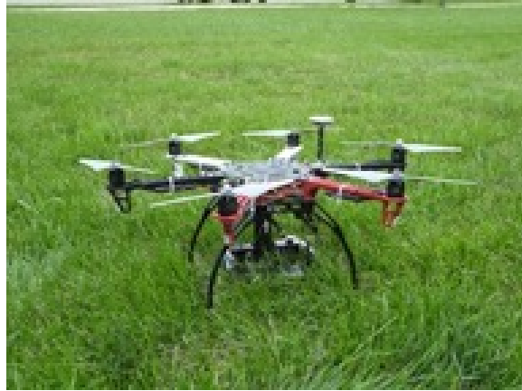
Fig. 8. A snapshot of Hexacopter-I UAV used for civil infrastructure inspection (Source: InfraDrone LLC)
